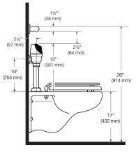
Per the ADA Guildlines (section 604.9.4) it is recommended that the grab bars be split or shifted to the wide side of the stall. If grab bars must be present over the valve, use the alternate ADA installation as shown to the right.
