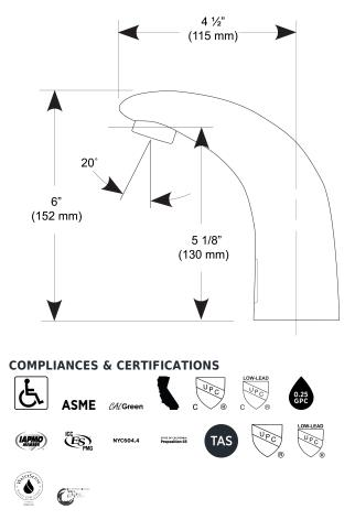
(ADA Compliant, ASME A112.18.1 Compliant, CalGreen Compliant, CEC Compliant, cUPC Certified, cUPC Low Lead Compliant, GPC 0.25 or less, IAPMO, NSF-61, NYC604.4, Proposition 65, TAS, UPC Certified, UPC Low Lead Compliant, WaterSense Listed, WELL Building Standard)
