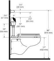
WHEN INSTALLING IN A HANDICAP STALL: Per the ADA Guildlines (section 604.9.4) it is recommended that the grab bars be
