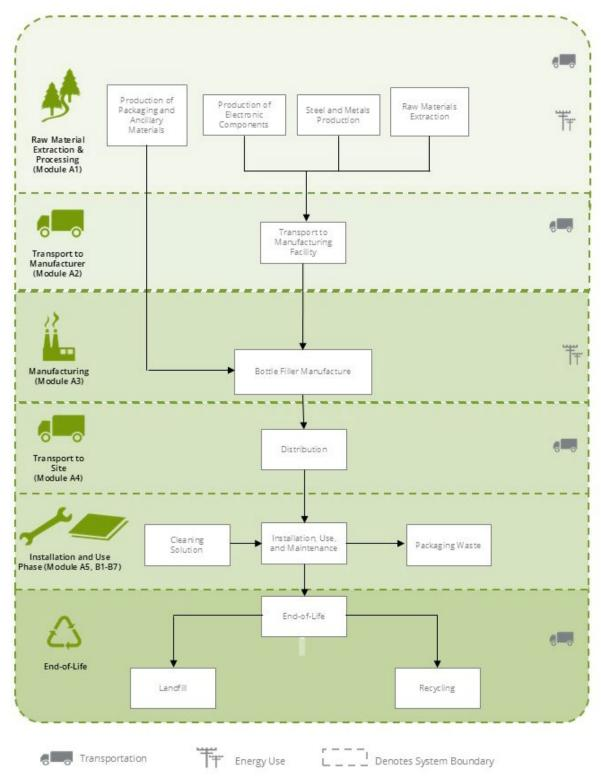
**Figure 1.** Flow diagram for the Sloan DropSpot™ Bottle Fillers.
