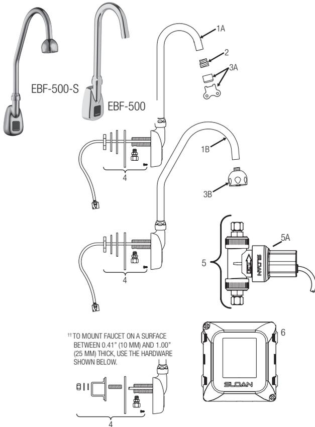
TO MOUNT FAUCET ON A SURFACE BETWEEN 0.41" (10 MM) AND 1.00" (25 MM) THICK, USE THE HARDWARE SHOWN BELOW.
