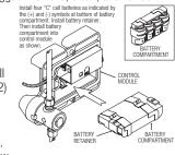
Remove the cover of the control module by unscrewing the four (4) cover screws located at the center of each side.
