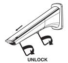
Rotate solenoid assembly counter-clockwise through a  $45^{\circ}$  angle.
