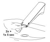
Cover IR clic until LED flashes RED 4 times - hold IR clic on until LED flashes 1 time to 8 times from minimum to maximum range. See diagram below. Release when requested range is reached.
