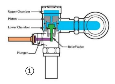
Incoming pressure to the upper chamber seals the piston down over the main seat
