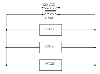
One EL-386 Transformer serves one (1) Optima Closet/Urinal Flushometer. One EL-451 Transformer serves up to eight (8) Optima Closet/Urinal Flushometers. 18 gauge wire (not supplied) required from transformer to flushometers.
