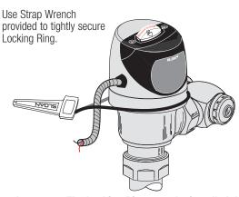
Important: The Locking Ring must be installed down past the valve body threads by at least one thread. If difficulty is experienced installing the Locking Ring, turn the Locking Ring back and forth, each time working it further down the threads. The Locking Ring will act as a thread chaser in the event there has been a build-up of matter on the threads of the old valve body.
