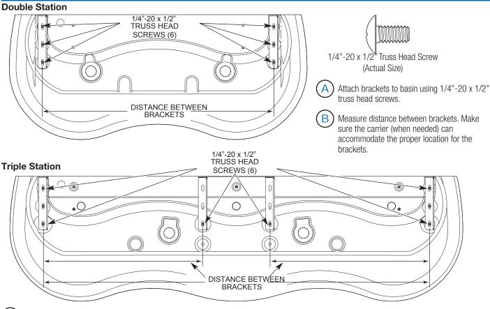
(C) Determine the appropriate location for the holes to secure the brackets to the wall. Use the following dimensions as a reference.
