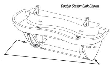
Replace End Caps. Insert the screw located on the inside of the Cap into the enlarged hole of the Frame. Then slide the Cap into place. Loosely install the two front screws. Slide End Cap UP to eliminate any gap between the End Cap and Basin. Tighten the inside screw securely. Lastly, tighten the two front screws securely. Follow the same procedure for the second End Cap.
