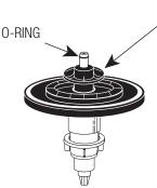
REGULATOR (MUST BE INSTALLED PAST O-RING)
