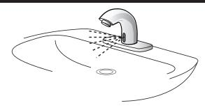
2. When hands are removed, the water flow should stop.
