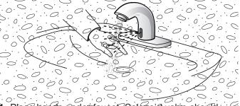
1. Place hands under faucet. Solenoid valve should "click," LED in sensor window should blink once and water should flow from the spout.
