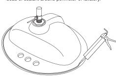
• Carefully align and lower the lavatory into place. Press evenly and firmly into position. Use a water dampened finger to smooth out any sealant around perimeter of lavatory. Allow sealant to set before connecting supply lines and waste pipes.
