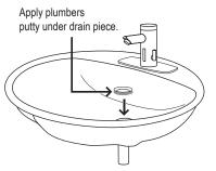
• Use plumbers putty on the underside of the drain to ensure a watertight seal as required. After tightening the drain assembly, remove excess putty that has squeezed out.
